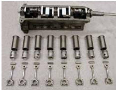
*Inside the straight eight engines are all the correct parts custom machined to scale from steel, cast iron and aluminium. Here we see the block and crankshaft at the top. Arrayed below the block are the cast iron cylinder sleeves, pistons, wrist pins and assembled connecting rods.*
