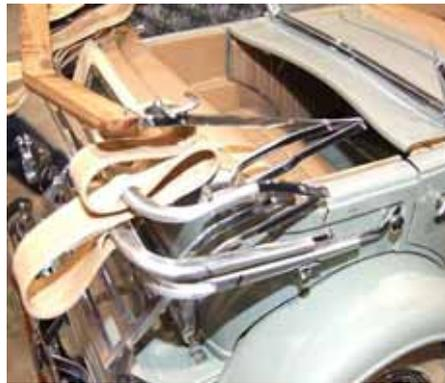
*The complicated convertible top mechanism is shown in the lowered position before the canvas top material was installed.*
