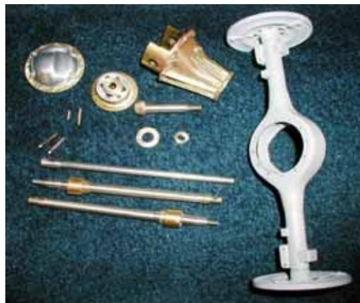
*The gears inside the differential will never be seen by anyone, but Lou cut them as actual hypoid gears like the real one rather than machining simpler*
