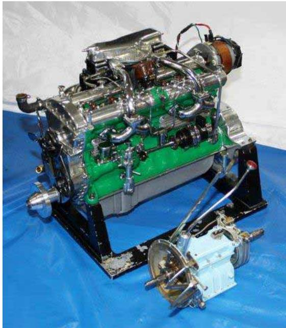
*Here is the engine removed from the model and sitting on its test stand. The transmission is in the foreground.*
