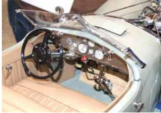
*This is the dashboard and interior with the body primed but not yet painted. Note the detailed instruments and engine-turned finish on the dash.*
