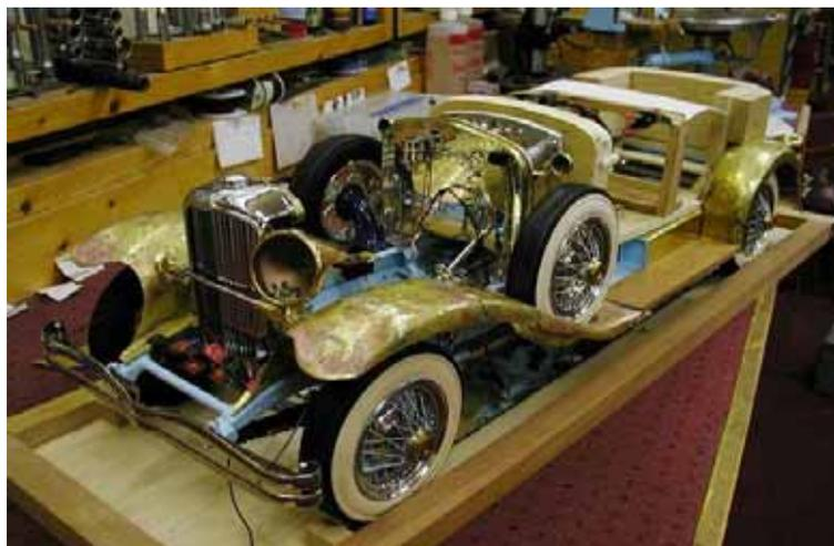
*The bodywork is all metal, not fiberglass. Here is the car in Lou's shop before the brass coachwork was primed or painted. Lou is not adverse to remaking a part that doesn't meet his standards. He started over on the especially difficult brass radiator shell nine times.*
